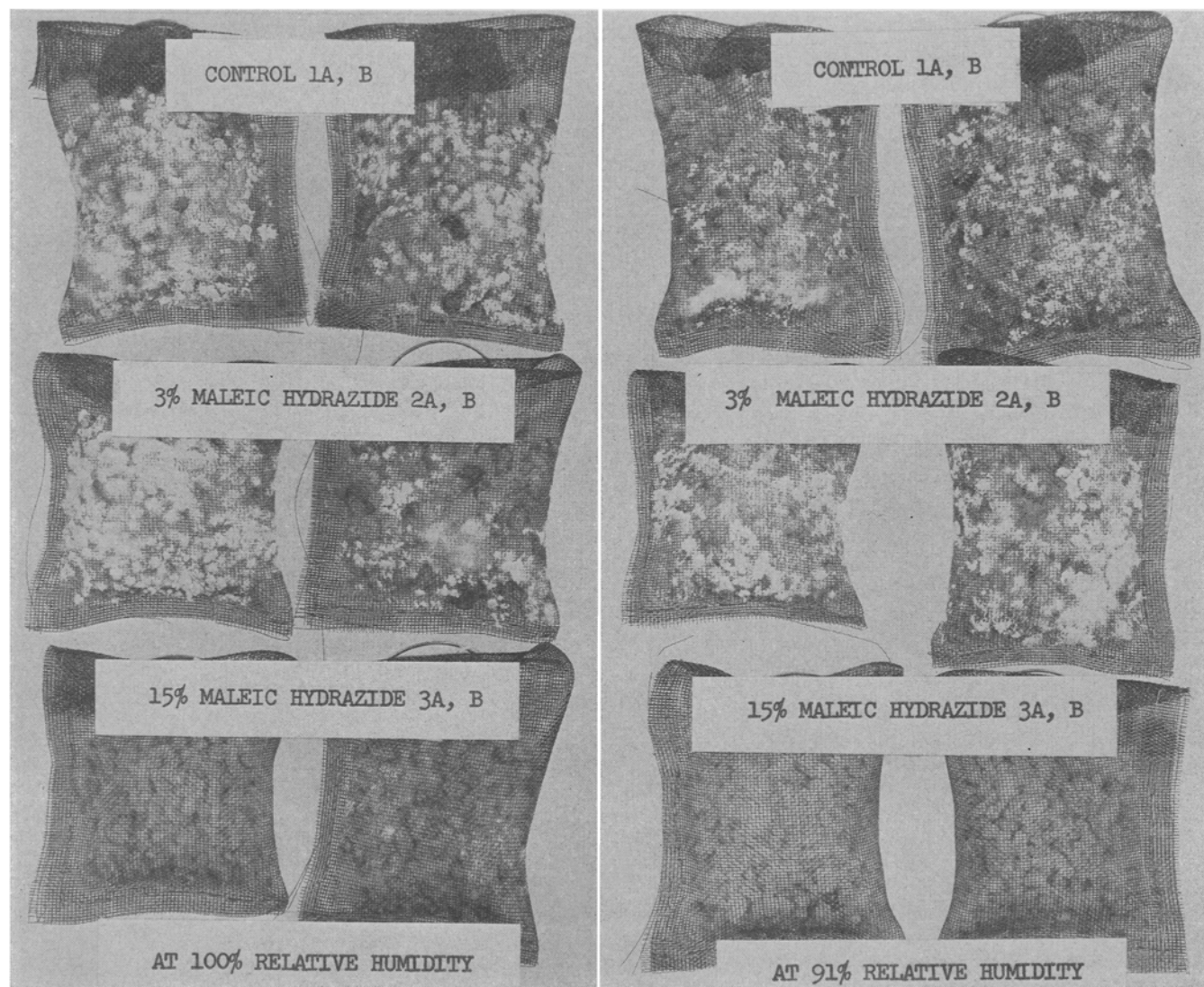
FIG. 1. Effect of maleic hydrazide sprayed on cotton plants at defoliation (A) and 16 days prior to defoliation (B) on the growth of mold on the harvested seed stored for 7 months at 78°F. and 100% R. H. (left) and 91% R. H. (right).
